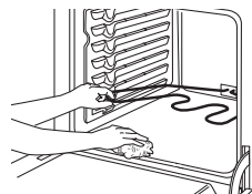
Gently lift the bake element
